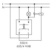
Single pole push buttons no contact with feedback signal
