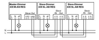
Circuit arrangement B: Combined switching of master and slave dimmers
