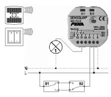
Actuation by presence detector/transmitter and existing electrical installation
