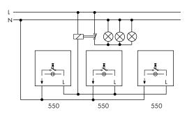
Staircase lighting (button-operated zero control)
