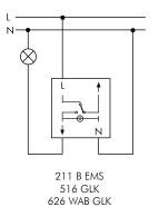
Two-way control switches as 1 pole on/off switches
