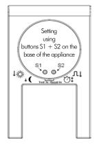
Range 120° Appliances: 10 m Switching capacity max. 1000 W
