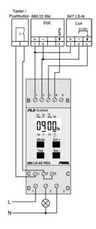
Function 1: Automatic ON and OFF triggered by motion detector - daylight-dependent. External light sensor in use; brightness is 1st priority
