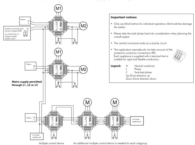
The application example shown here shows "single drive operation". The drives can also be operated in "dual drive operation" model.
