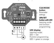
Easyclick flush-mounted JR receiver Plus, 2-channel 452 FU-EP JR o.T.
