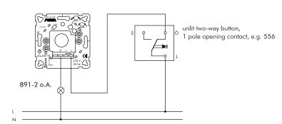
The automatic switch is turned on for the pre-selected time by pressing the button.
