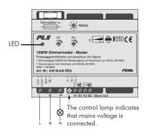
Basic circuit diagram for individual operation of the dimmer with power connection  $230\,V\!\!\sim\!/\,50\text{-}60\,Hz$  at terminal L, N and load on the terminal X.
