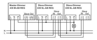
Circuit arrangement C: Combined switching of master and slave dimmers
