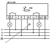
Button for switching the lighting on/off manually
