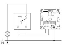
Two-way switching of the dimming function on the dimmer only
