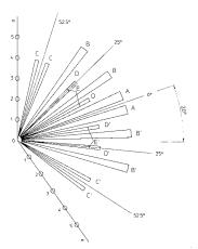
Bird's view sensor zones, sensor at a lateral angle of  $20^\circ$ , for mounting next to doors. Mounting height 0.80-1.20 m.
