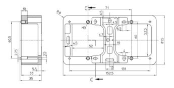
Hole pattern for mounting the dual housing
