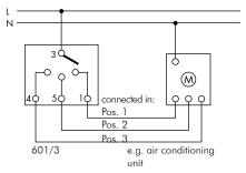
3 pole step switches, with 0 position
