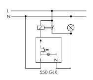
Single pole push buttons, no contact with feedback signal
