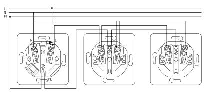
Additional earthing contact sockets can be protected by simply wiring through, as shown on the wiring diagram!
