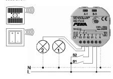
Actuation by presence detector/transmitter and substation S1 and S2 (button or switch)
