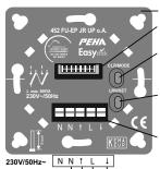
Mounting plate Jack for touch adapter CIR/MODE button with LED Delete all
