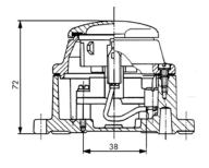
Earthing contact socket with flap, surface-mounted
