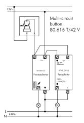
Remote control switch combined with remote control touch dimmer
