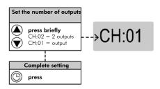
Note: The setting is activated automatically when the system is commissioned for the first time.
