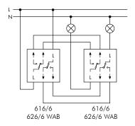
Dual multiway switching with two dual two-way switches
