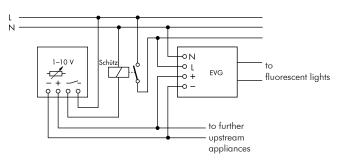
Upstream appliances have high levels of peak currents when switched on. A power relay must be used, if more than 5 upstream appliances need to be switched. Consult the technical specifications of the upstream appliances.
