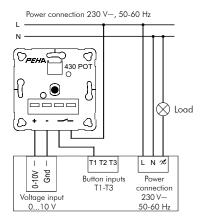
The dimming of the load is controlled using an externally connected potentiometer, e.g. PEHA's electronic potentiometer 430 POT on the terminals "0...10 V" and GND of the universal dimmer. (see switching example)
