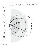
Ultrasound range 7,5 6 4,5 3 1,5 0 1,5 3 4,5 6 7,5 9 m 7.5 Minor movement 4,5 Major movement 3 1,5 Infrared range 0 Minor movement 1,5 3 Major movement 4,5 6 Figures in metres
