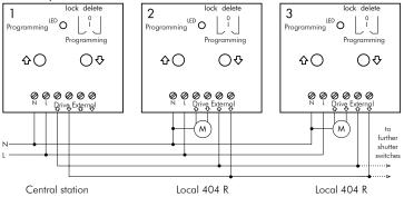
All shutter switches must be connected in the same phase!
