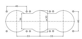
Cut-out for built-in socket 1 x triple, 703 Do
