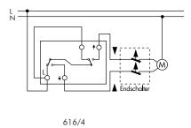
Blind (shutter) switches with electrical interlock
