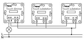
Connection diagram for controlling substations instead of using existing cross wiring
