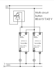
Remote control touch dimmer operation of 2 lighting points with two 879 TR EV/12
