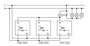
Staircase lighting (button-operated zero control)
