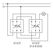
Multiway switching with 2 pole two-way switches
